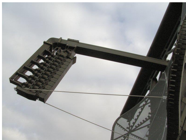
Figure 19: An arrangement of twelve feed horns at the antenna of the radar set ASR 910 achieves a stacked beam cosecant squared pattern
