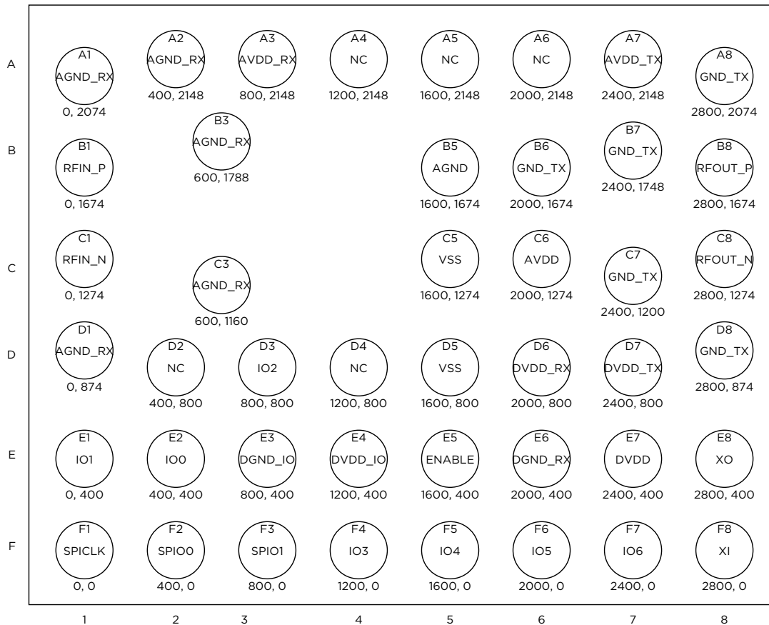
Figure 2.1. Top view footprint (coordinates in micrometers)
