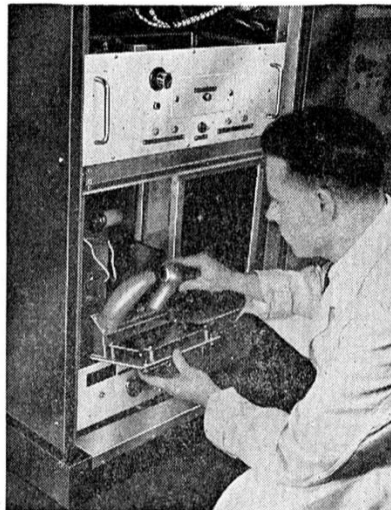
Accessibility: The magnetron, like all major units, is readily accessible.
