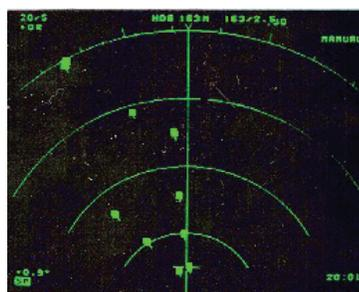
The Skin Paint mode provides a clutter-free display and automatic tilt and gain operation.
