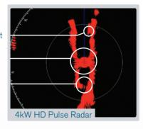
4 kW HD pulse radar can not discriminate the moored vessel from shoreline, "main bang" obscures width of channel.
