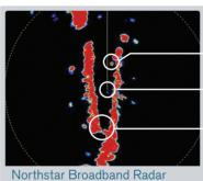
Broadband Radar clearly defines this narrow 35-meter channel, showing a small vessel moored near shore and a small footbridge.
