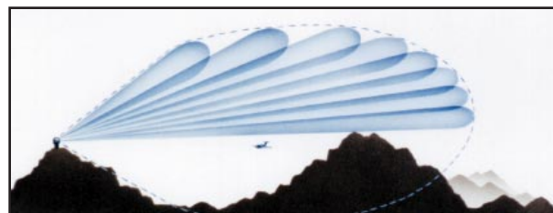
Performance gaps are possible with Stacked Beam Architecture.
