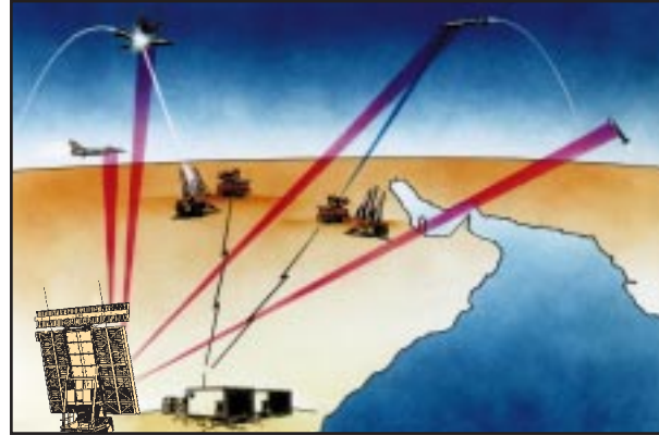
The FPS-117 has optional air and missile defense capability.
