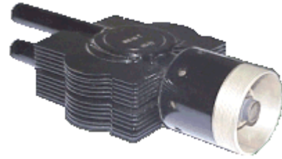
Figure 9: Magnetron MI 29Г of the old Russian Radar "Bar Lock"
