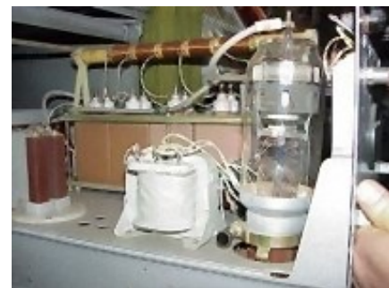
Figure 6: ancient modulator (Spoon Rest D) showing all components of a modulator
