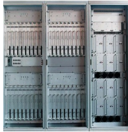
Figure 13: Solid state amplifier of the ATC-radar ASR-E (Manufacturer: EADS)
