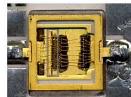
Figure 15: GaAs-MeSFET Transistor in MMIC Technology
