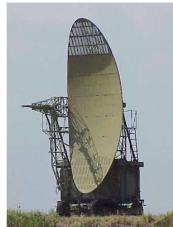
Figure 14: Typical antenna of a height-finder using an offset antenna forming a fan beam
