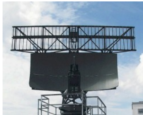
Figure 2: A monopulse secondary surveillance radar antenna (looks like a lattice fence) mounted on top of an antenna of a primary radar (parabolic reflector)
