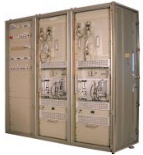
Dual electronics housed in EMC cabinets
