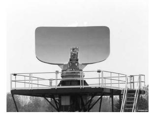
returns. Polarisation switching between Linear and Circular is provided on both low and high beams and a cross polarised output is available on both beams which can be used as a receive weather channel.
