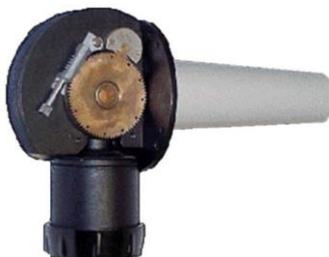
Figure 17: Magnetron M5114B of the ATC-radar ASR-910
