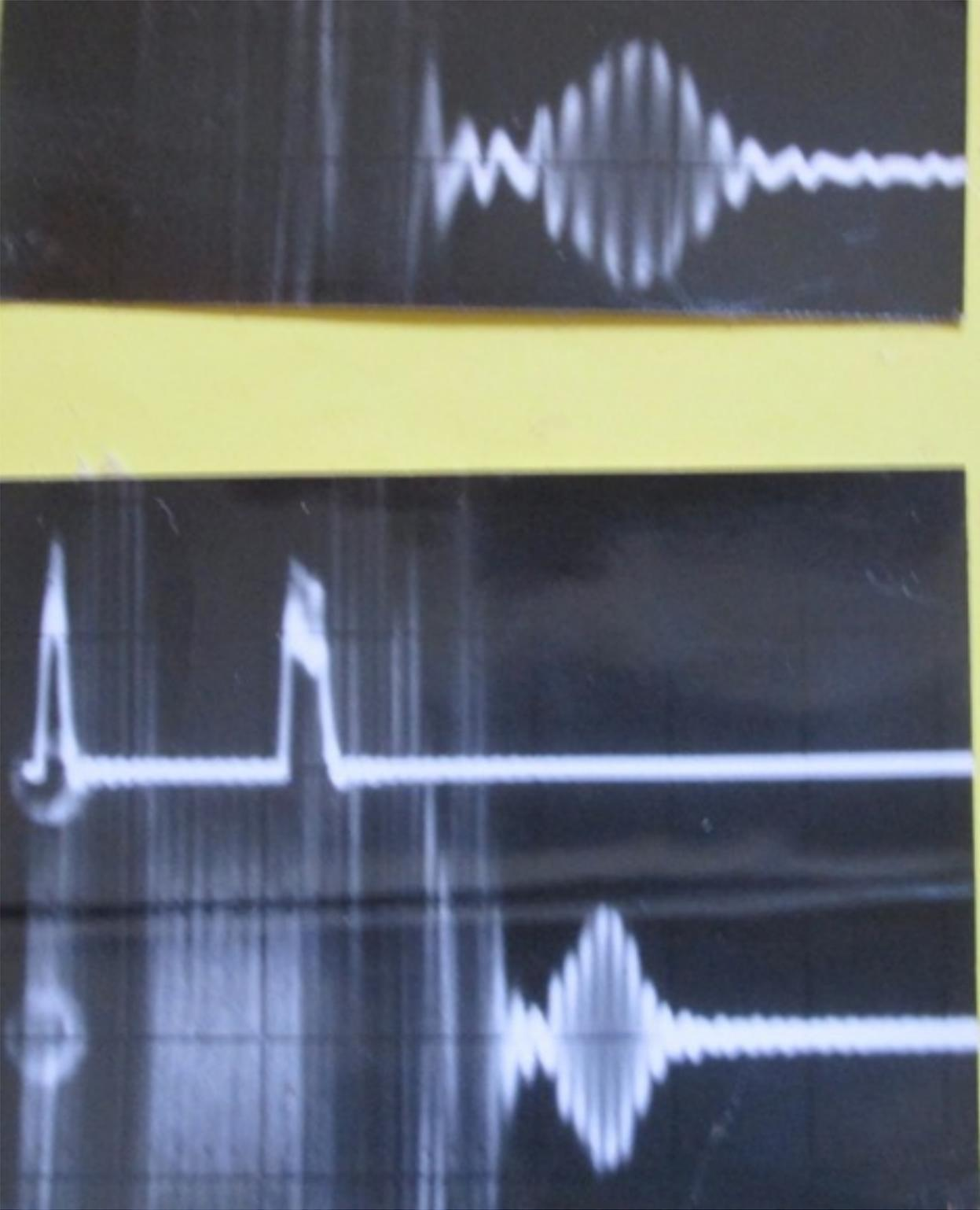
Figure 2b weak echo from Biphenyl radical in Boric acid glass , sample supplied by Professor J. Schmidt of Leiden Univeristy Huygens Laboratory.
