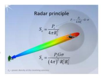
The receiving antenna of the radar is located in the environment of this power density. This antenna also has an effective antenna area, which is formed by the geometric area A multiplied by a matching factor  $K_a$  containing the efficiency. Together with the power density Se applied at this location, this gives the received power of the antenna  $P_e$ .
