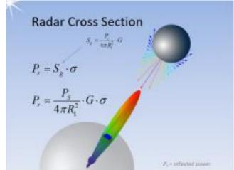
Simplified: the reflecting object can again be considered a radiator based on the reflected power. The reflected power then becomes the radiated power (from the reflector).
