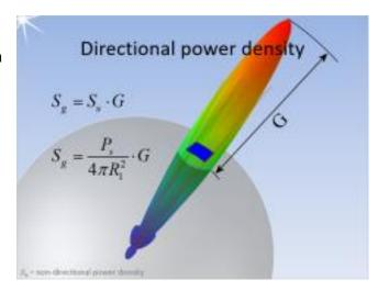
Now it depends on how large the effective reflection area of this object is, i.e. how much of this power density is backscattered.
