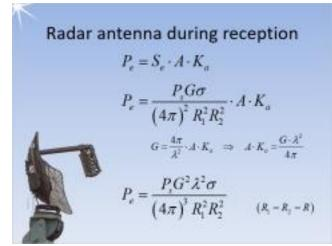
another equation that arises when deriving the antenna gain of an antenna. If this equation is rearranged to  $A \cdot K_a$ , we can substitute this term. As a result, the  $4\pi$  now appears to the third power and the wavelength lambda appears in the equation. The antenna gain G is now raised to the square: this is also logical because this gain acts on both transmission and reception.
