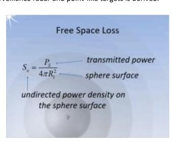
approximately the speed of light, the spherical surface becomes larger and larger. The power density per unit area on this spherical surface results from the ratio of a small unit area to the total surface area of the sphere, multiplied by the transmitting power.
