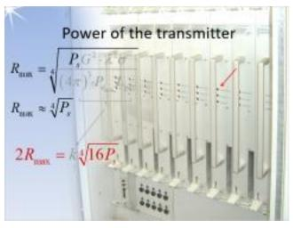
picture shows power amplifier modules of the transmitter of an air traffic control radar. The power amplifier stage consists of up to 32 such modules. If one of these modules fails, a remaining range of 99.2% (the fourth root of 31/32) remains. This would not be noticeable on the radar display. But the technician sees that the red LEDs "module error" and "module off" light up and can change this module even during operation.
