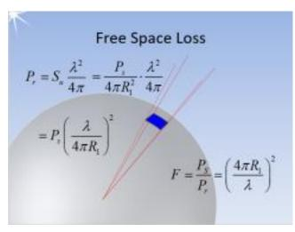
We have already seen the undirected power density  $S_u$  as the transmitted power distributed on the surface of the sphere, and we use this expression here.
